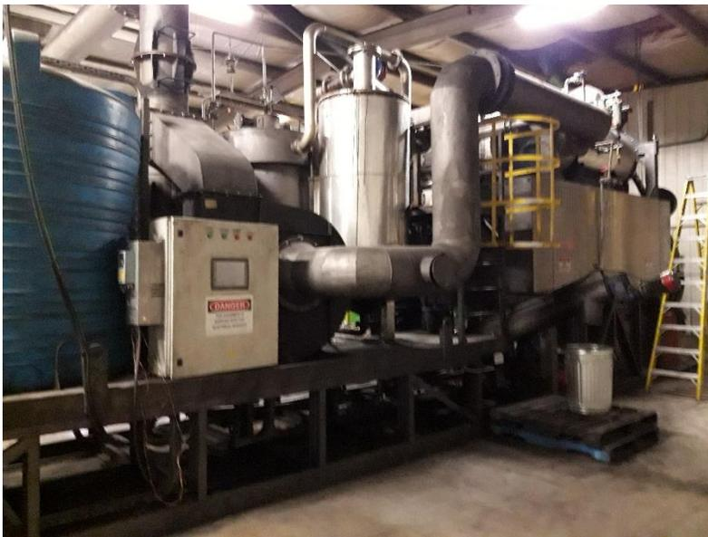
This was accomplished by incorporating a more advanced physical activation system incorporating the use of super-heated steam (temperature approx. 500C). Not only did our Technical team address this issue but they also engineered a novel way of creating this super-heated steam using the heated thermal chamber as a source for super heating the steam. Subsequently, further improvements were developed involving a thermal chamber containing 3 reactor tubes, each
